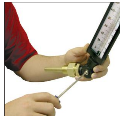
Tighten screw (A) to secure the angle.
