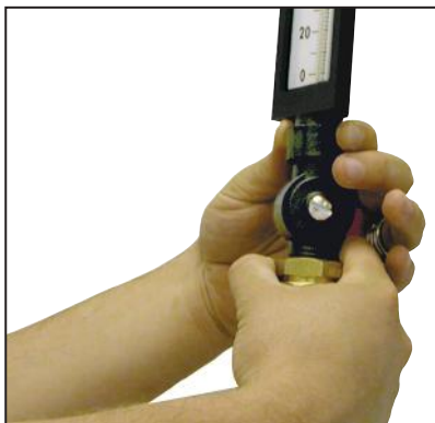
Rotate locking nut by hand.
